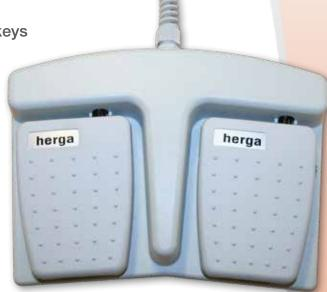
The 6225-0020 is a 2 pedal USB footswitch supplied with grey pedals and base. With DIP switches for customer programming, the switch is supplied with 2.5 metre cable as an IPX2 rated assembly for operation from a 20 mA 5V DC supply.
